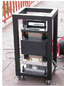
Figure 6-2: Electromagnetic shaker for civil engineering applications. Vertical mounting.
