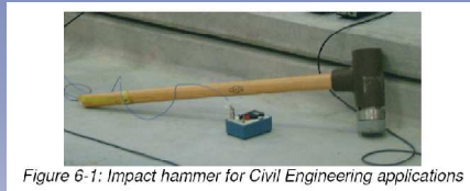
Figure 6-1: Impact hammer for Civil Engineering applications
